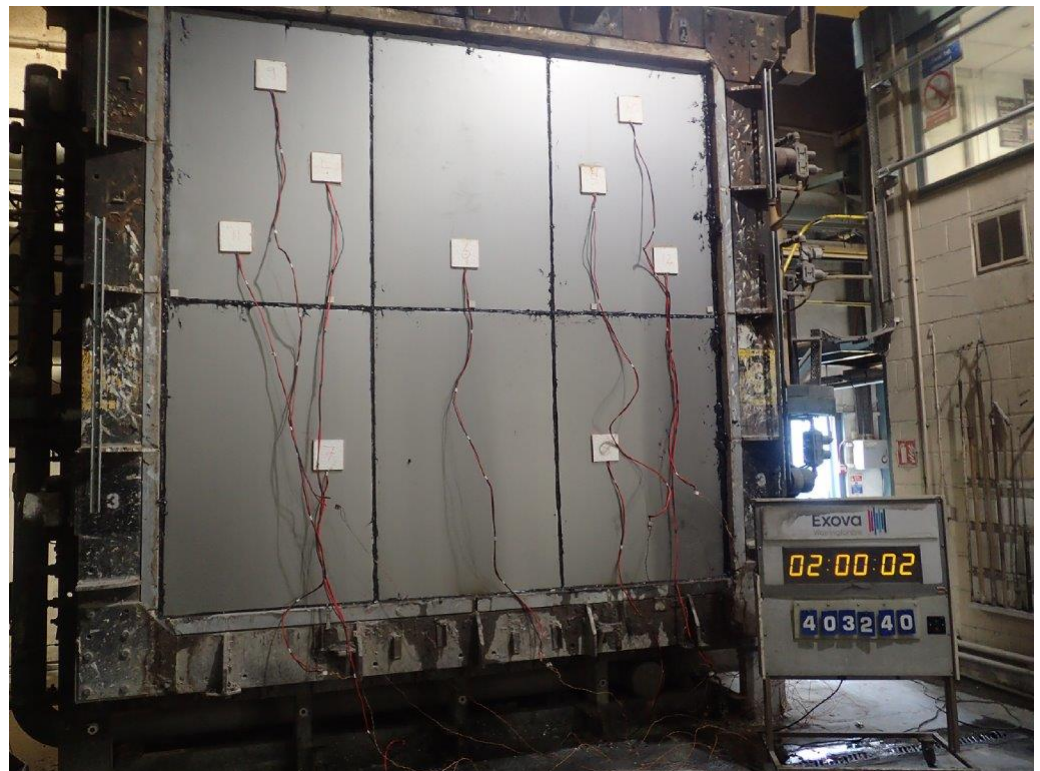
The unexposed face of the specimen after 120 minutes of testing.
