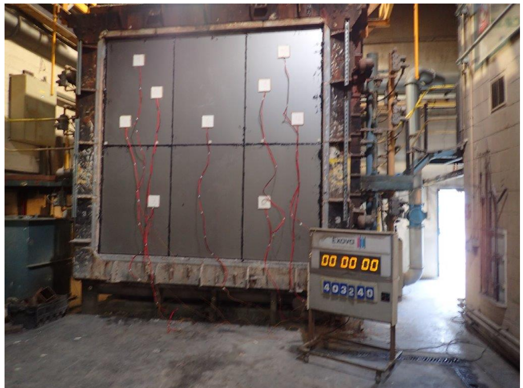
The unexposed face of the specimen prior to testing.
