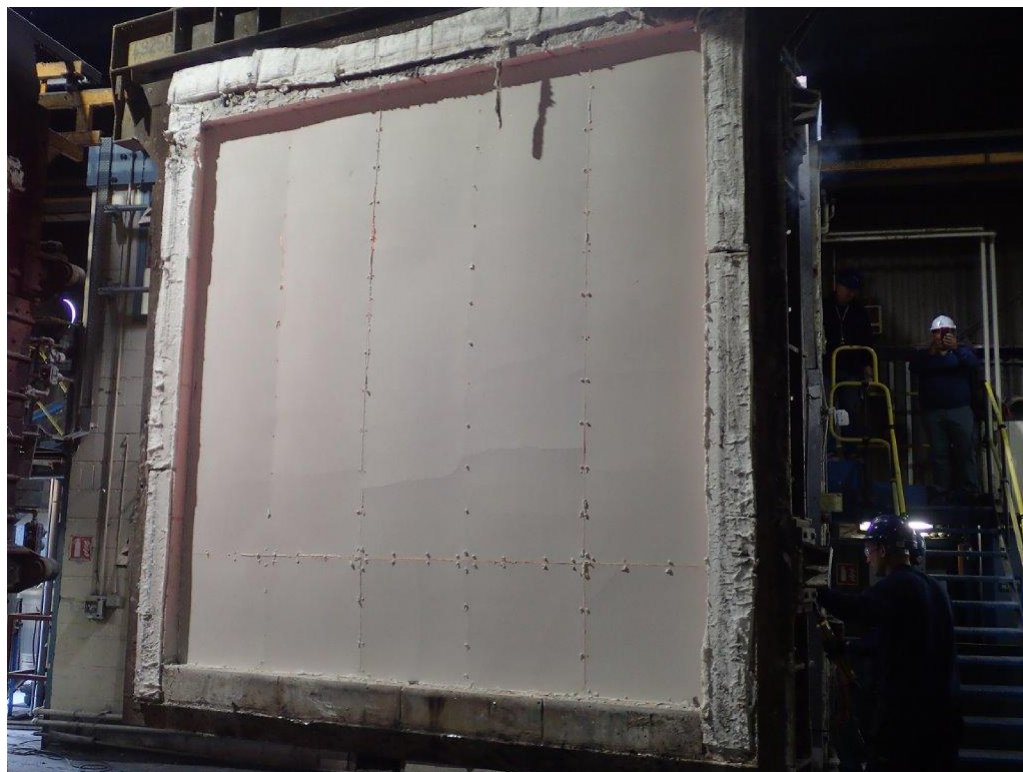
The exposed face of the specimen immediately after testing.
