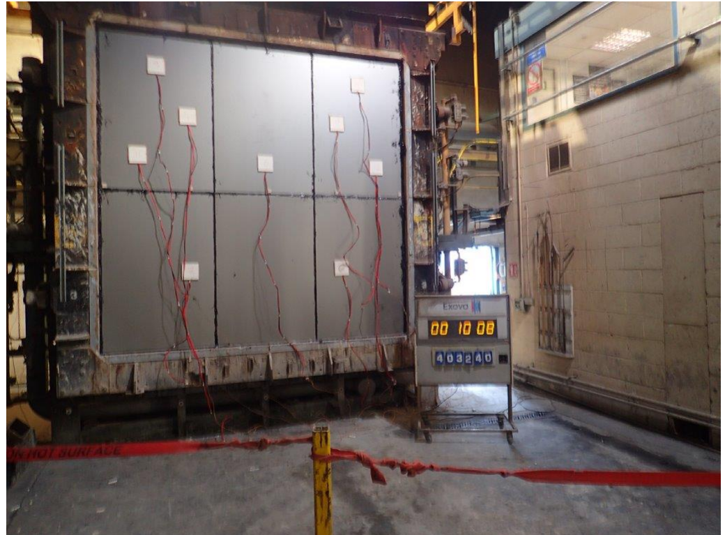
The unexposed face of the specimen after a test duration of 10 minutes.
