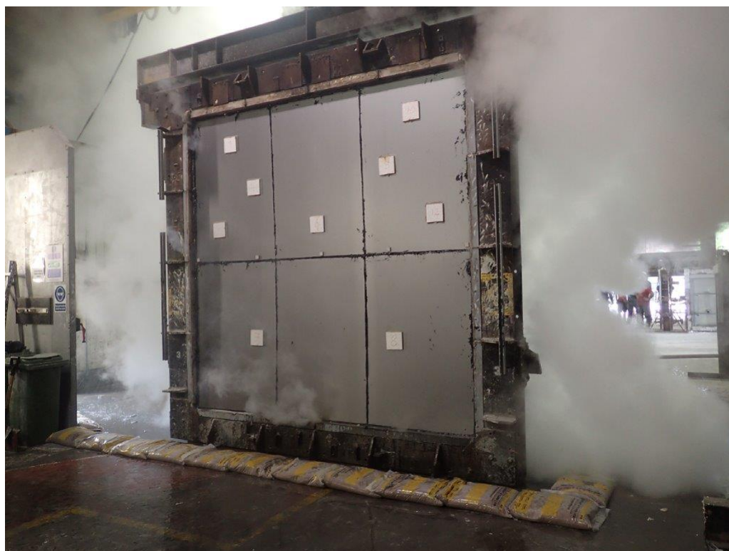
The unexposed face of the assembly during the hose stream test.
