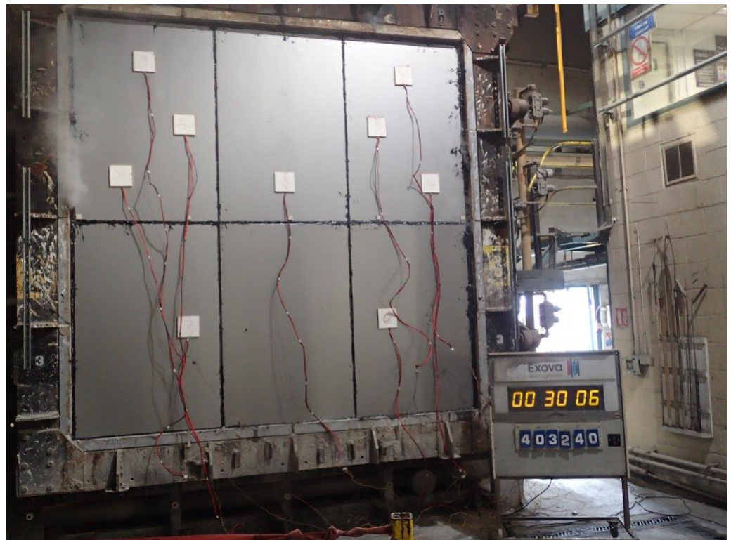
The unexposed face of the specimen after a test duration of 30 minutes.
